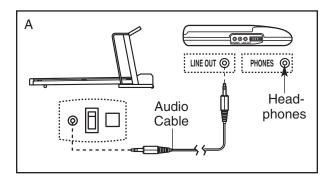
B. Plug one end of the audio cable into the jack on the front of the Incline Trainer near the power cord. Plug the other end of the cable into a 3.5mm Y-adapter (available at electronics stores). Plug the Y-adapter into the PHONES jack on your CD player. Plug your headphones into the other side of the Y-adapter.
